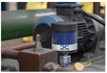
To keep machinery from building up too much pressure, equipment OEM's include **vent caps** on the fill port to allow expanded air to escape. These **simple caps** do let the air out of the equipment but these cannot prevent small dirt particles and moisture to enter into the equipment/tank which can damage bearings, gears & valves. Also these caps cause condensation of the moistures that contaminates the oil further.
