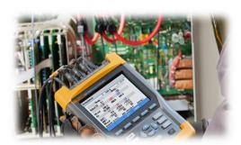
include voltage, amperage, frequency, dips (sags) and swells in voltage values, power factor, harmonic currents, and the resulting distortion and crest factor, power and energy, voltage and current unbalance, inrush current values, and light flicker. If an analyzer measures and records such basic parameters, you can address most power quality issues successfully.
